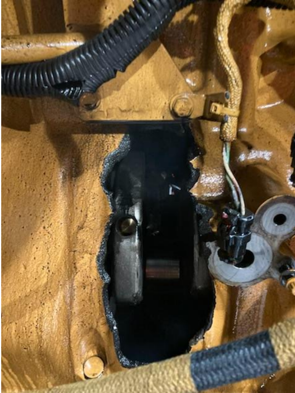
Figure A-2: Hole in the Engine Block where the Connecting Rod was Ejected from the Engine
